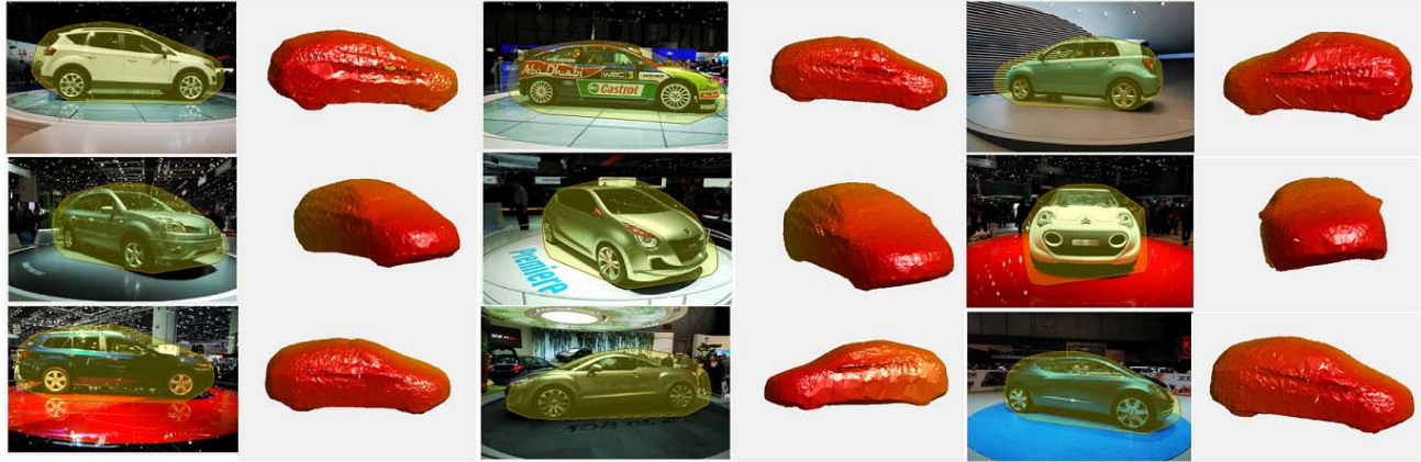
Figure 4: Qualitative results. Left : Test images overlaid with the projection (2D convex hull) of the estimated shape and viewpoint. Right : Full 3D reconstruction of the test object instance obtained by deforming basis shapes (meshes) using estimated shape parameters rotated to the estimated pose.
